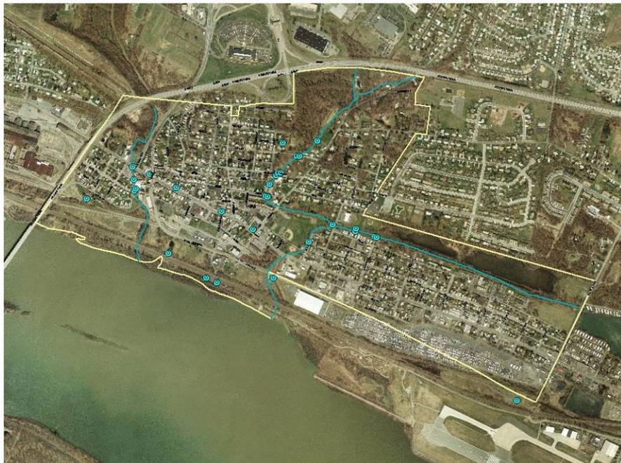
Aerial view of mapped stormwater outfalls (light blue points) and streams (light blue lines)
