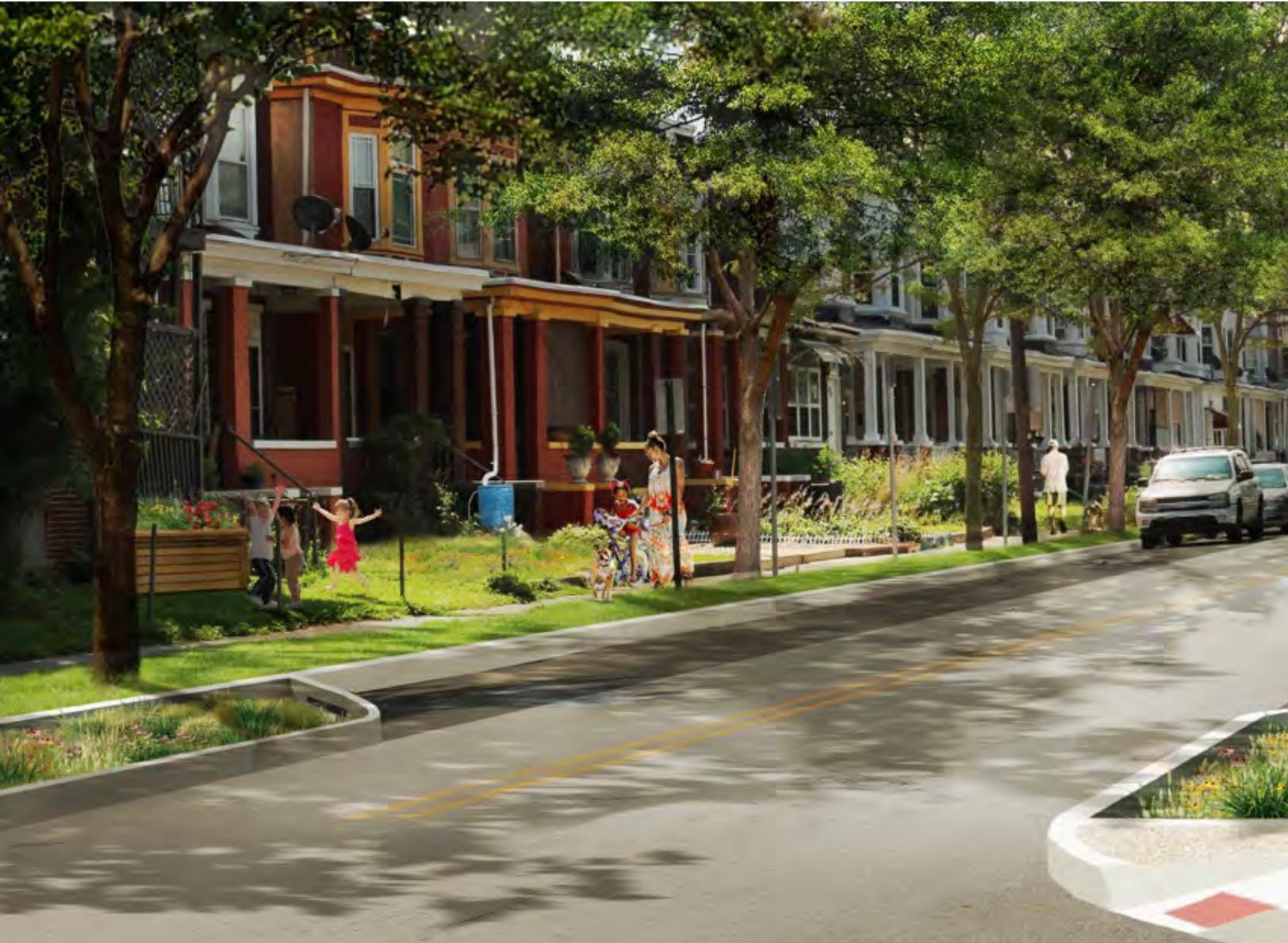
a more welcoming pedestrian environment. A small rain garden, flow-through planter, and rain barrel manage stormwater runoff from roofs on the eastern side of the street.
