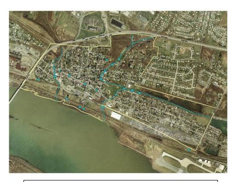
Aerial view of mapped stormwater outfalls (light blue points) and streams (light blue lines)
