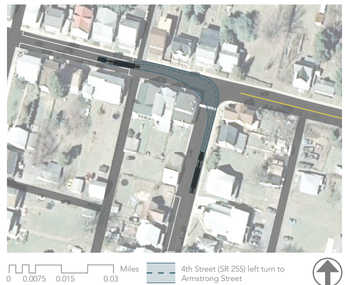
FIGURE 10: SR 225/Armstrong Street @ SR 225/4th Street Autoturn Swept Paths - New Turning Movements
