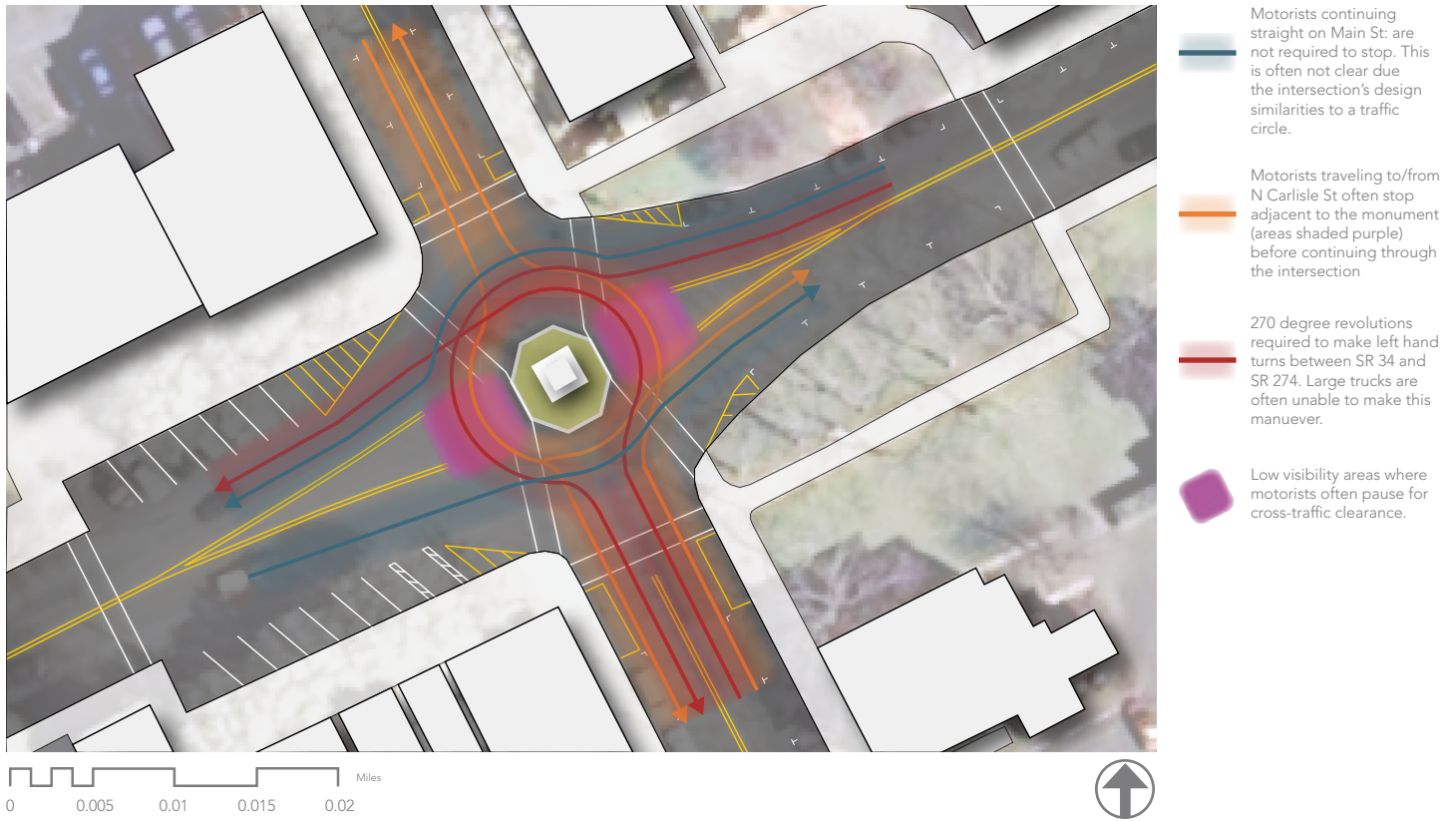
FIGURE 6: Autoturn Swept Path - 53' Trailer
