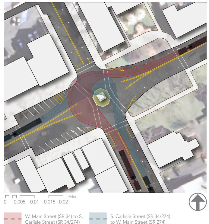
FIGURE 6: Autoturn Swept Path - 53' Trailer
