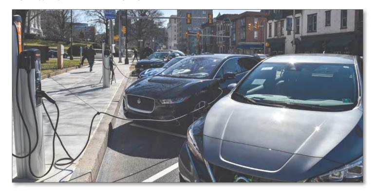
EVSE (electric vehicle supply equipment) unit and wiring capable of handling the voltage. They provide 10 to 25 miles per hour of charge. Level 2 chargers are most sufficient for multi-unit dwellings, shopping malls, parking structures, business parks or anywhere people park for a few hours at a time.
